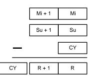
**Note** The DOUBLE 2's COMPLEMENT – NEGL(—) instruction can be used to convert binary data only, it cannot be used with BCD data.
